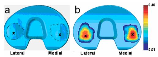
Comparison of experimental (a) and simulated (b) wear regions for a total knee replacement design after 5 million cycles of walking performed in a knee simulator machine. Xs indicate locations of maximum wear. Dotted lines in (a) indicate boundaries of experimental wear regions. Color bar in (b) indicates depth in millimeters of simulated wear regions.
