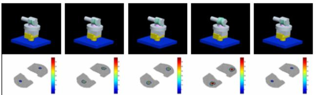
Animation strip of computer simulation of a knee simulator machine used to evaluate the wear performance of new knee replacement designs. Top row shows simulated motion of the knee design in the machine. Bottom row shows corresponding location and severity of contact as needed to predict the wear performance of the design.
