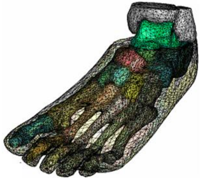
Subject-specific finite-element model of the foot.
