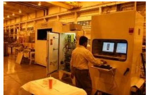
An operator inspects the images of an engine block in which pores were detected and makes the intelligent decision as to whether the engine block is indeed defective
