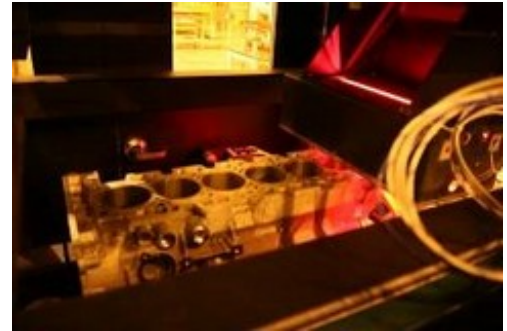
Engine block moves into the in-line porosity inspection station
