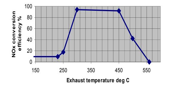
High NOx reduction efficiency within the catalyst temperature range
