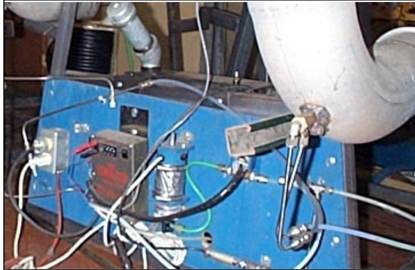
Figure 2-3. Reductant injection system for lean-NO x catalysts
