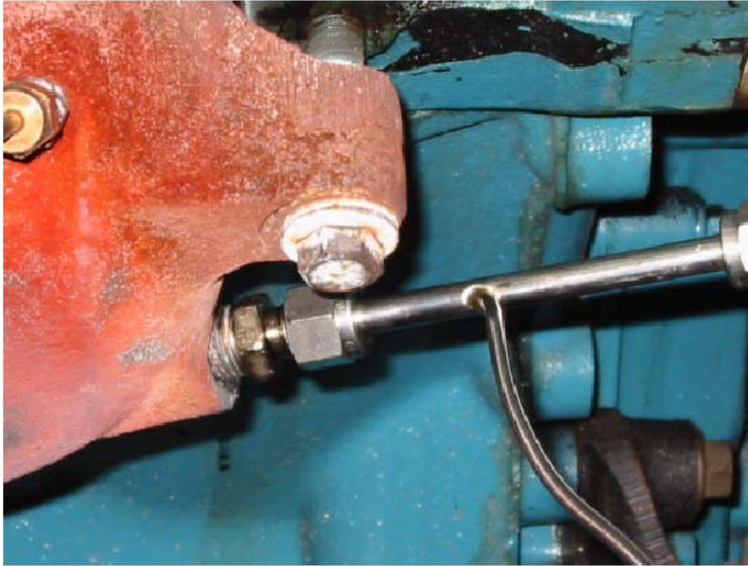
Figure C-2. Oil injector body attached to exhaust manifold.
