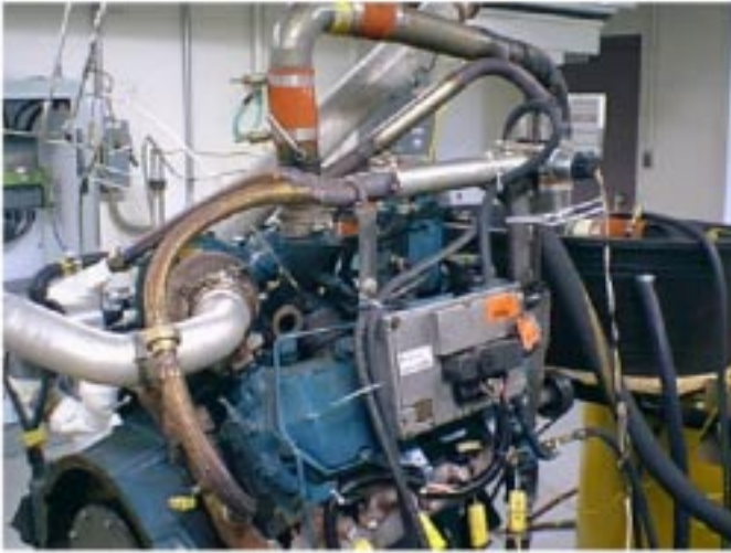
Additional hardware was installed in this engine to accommodate the exhaust gas recirculation system.
