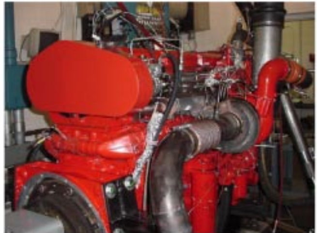
A Cummins ISX engine is shown in the test cell, where durability tests will be conducted.
