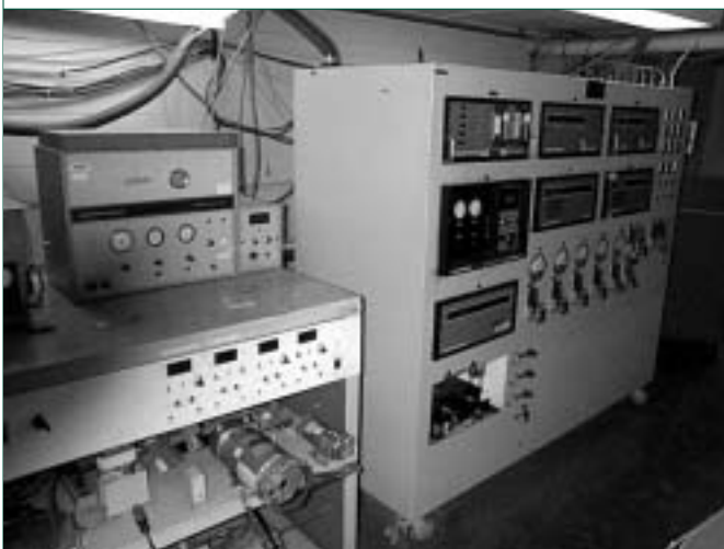
Emissions benches like this one at WVU were used to collect data during the tests.
