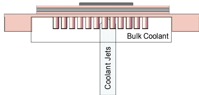
Surface area is a key parameter for enhancing heat transfer, enabling volume and cost reduction
