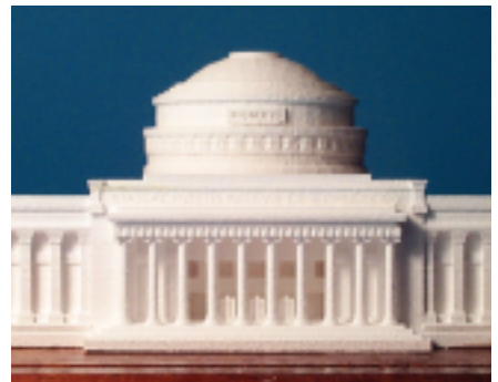
Model of MIT made by 3-D printing, a fabrication technique that builds parts layer by layer. An ink jet printer delivers a binder that selectively joins a powdered material that makes up each layer. About six inches long, the model was made from alumina powder with a binder of colloidal silica.
