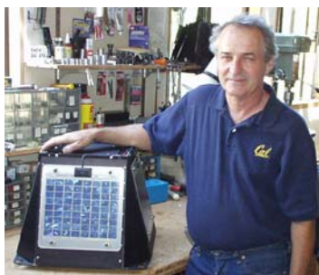
'Mini' Taisu under development for testing in 2003/04 Antarctic season: datalogger, Iridium modem. 15 kg. max
