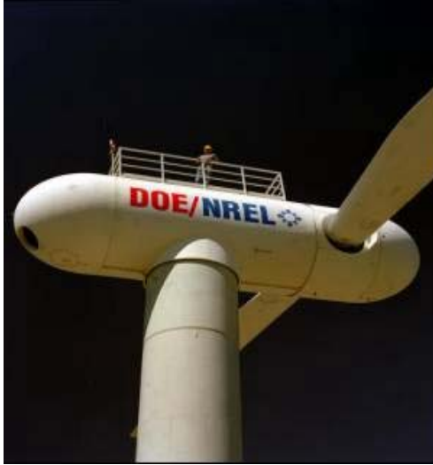
Figure 1. The controls advanced research turbine (CART).
