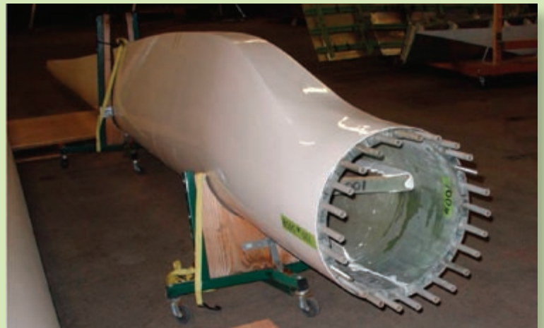
SNL produced a 9-m subscale blade in 2006 that demonstrates significant reductions in weight and costs while increasing strength.
