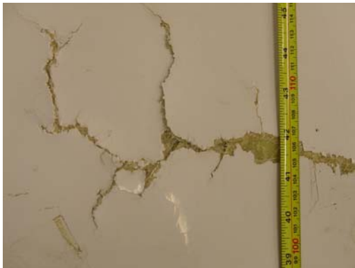
Figure 24: Crack near blade centerline on TX-100 blade.
