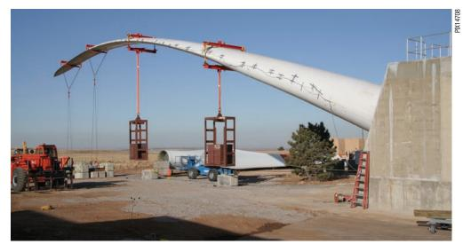
wind turbine models. NREL operates the only blade test facility in North America capable of performing full-scale testing of megawatt-scale wind turbine blades. Rapid growth in wind turbine size over the past two decades has outstripped the capabilities of this blade test facility, leaving the U.S. wind industry without a suitable means of testing blades for large land-based and offshore turbines.
