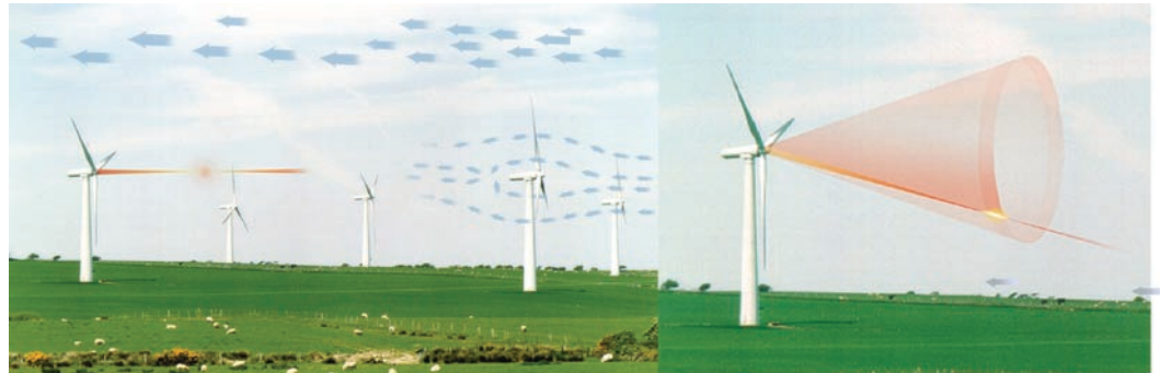
Examples of LIDAR scanning options, showing hub-mounted staring scheme and hub-mounted conical scan.
