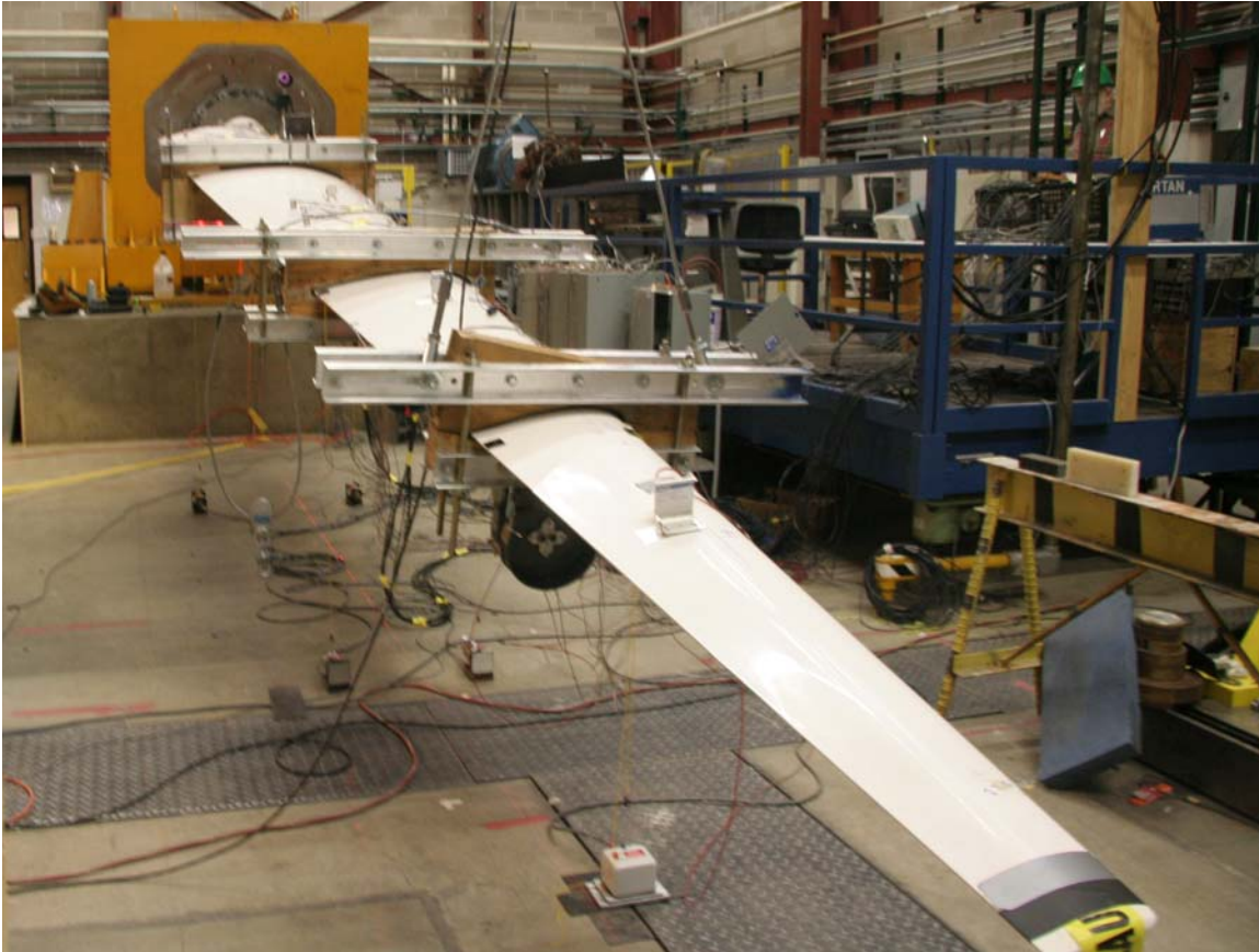
Figure 2. Blade static test
