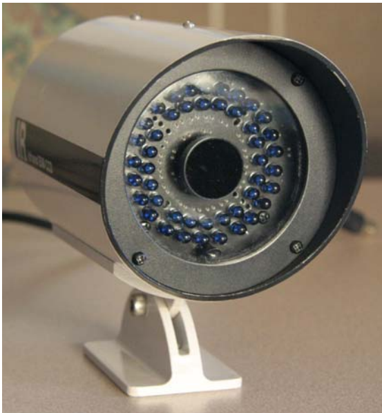
Figure 1. Security camera with infrared emitter and IR filter
