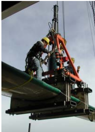
Figure 8: Installation of the NWTC B-REX fatigue testing system
