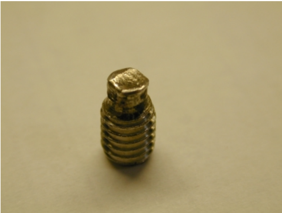
Figure 12: The setscrew. Note the wear on the top of the setscrew.
