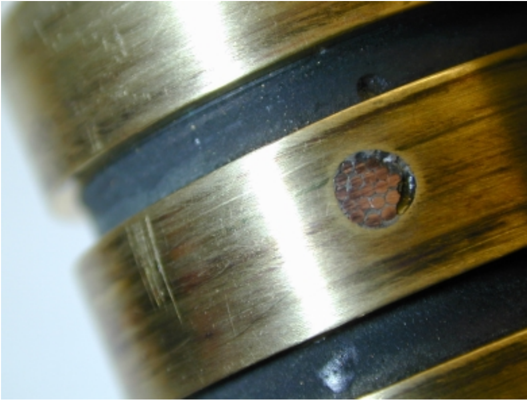
Figure 7: As a comparison a good connection on one of the other slip ring channels.
