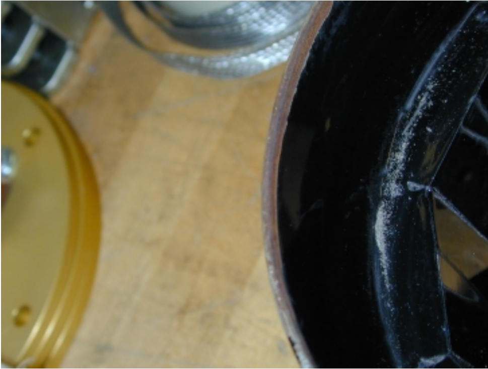
Figure 3: Wear on the edge of the magnet can
