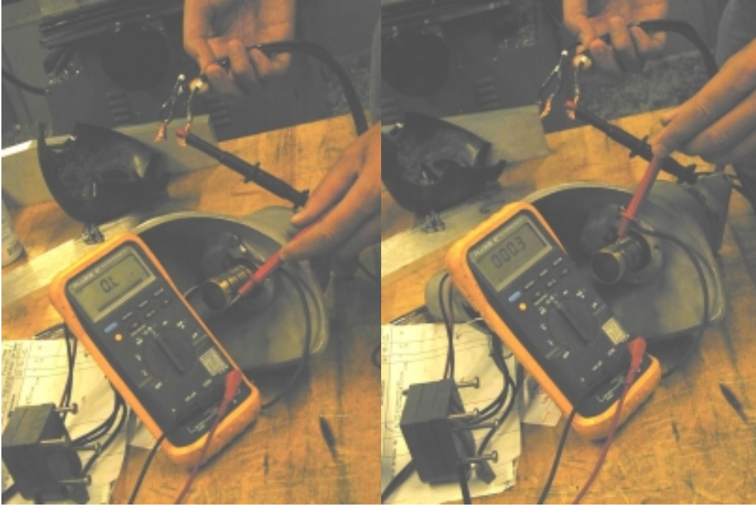
Figure 5: Left: measuring resistance between the slip ring race and the end of the wire, no contact. Right: Measuring resistance between one end of the wire and the wire end in the slip ring hole, connection.
