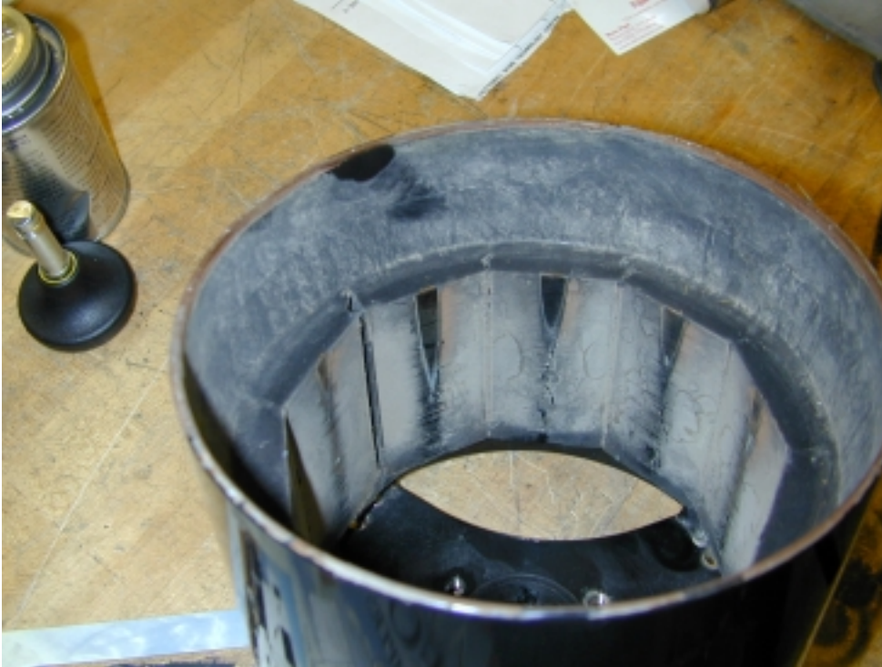
Figure 1: Signs of wear on the magnet can
