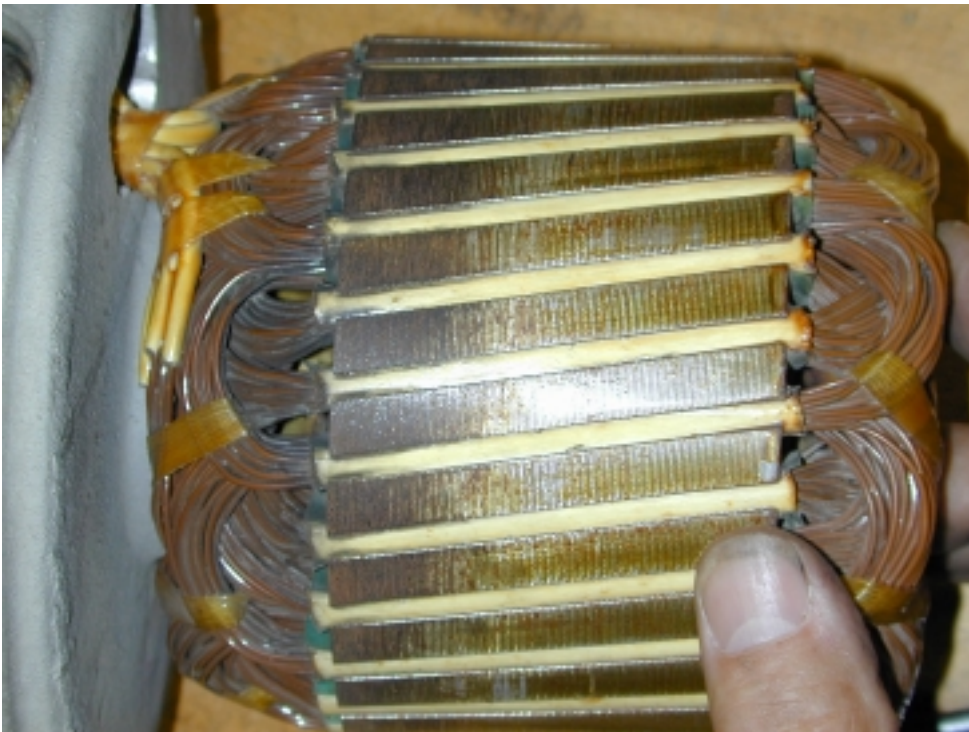
Figure 4: Windings on the downwind side (left) seem slightly decolorized compared to the windings on the up wind side (right). Further the brown areas on the left show where the magnets have been rubbing the stator lamination.
