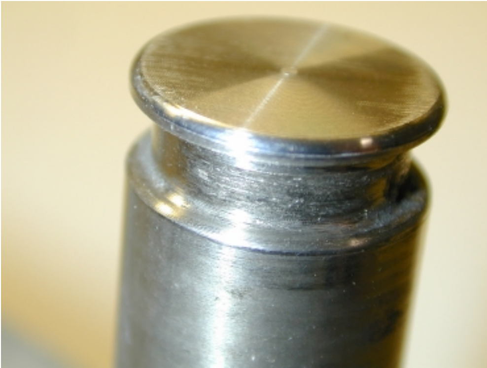
Figure 13: Close up of the groove in the pivot pin. Some wear caused by the setscrew is present.
