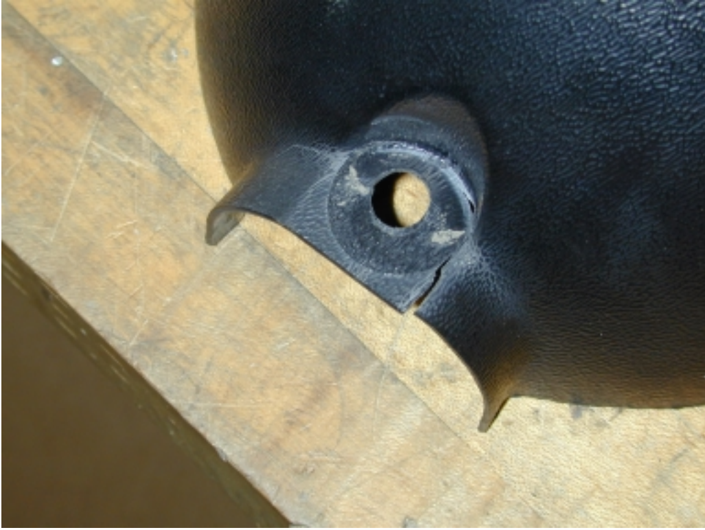
Figure 15: Close up of the nose cone. The holes are use by the fasteners connecting the nose cone to the hub.
