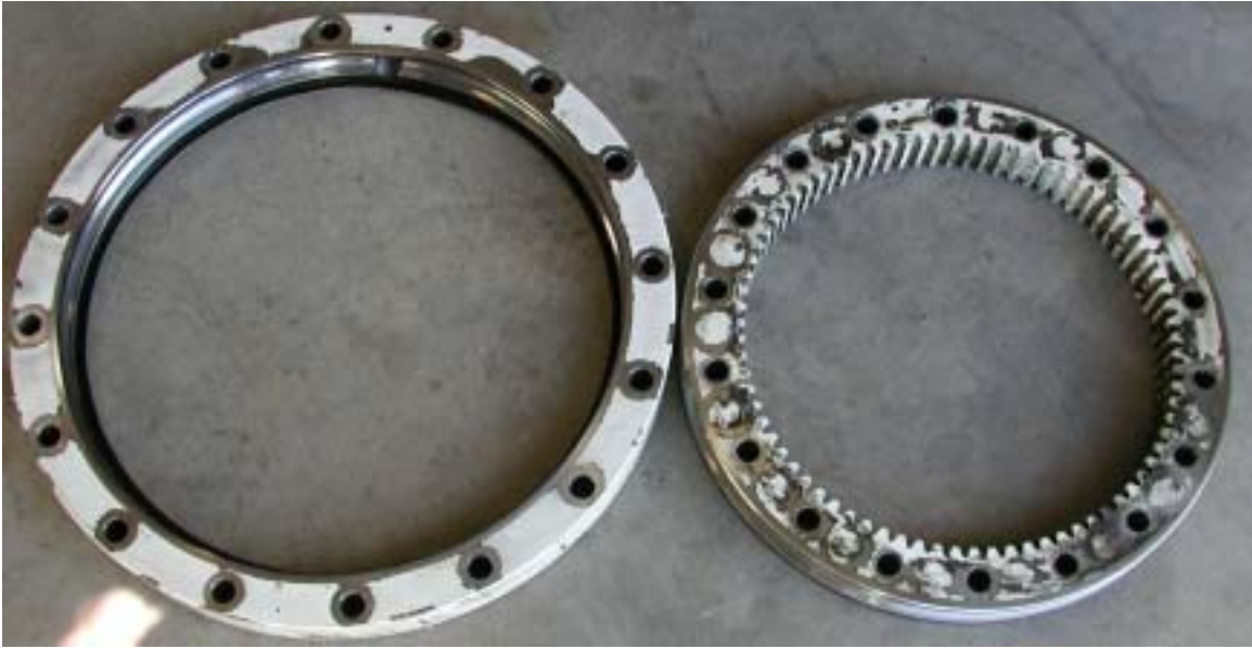
Figure B.4. The disassembled yaw bearing.
