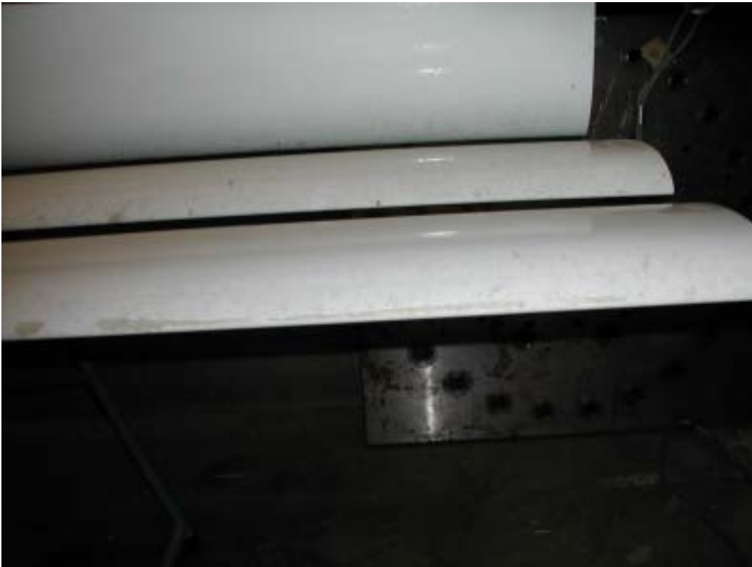
Figure D.3. Paint erosion on leading edge of blade 1.
