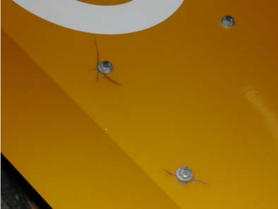
Figure D.6. Cracks near the downwind bolts on the tail vane.
