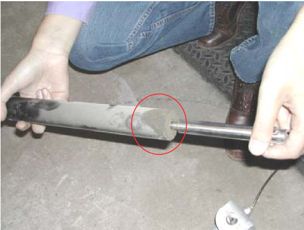
Figure D.13. The furl damper with some signs of leakage on the right side.
