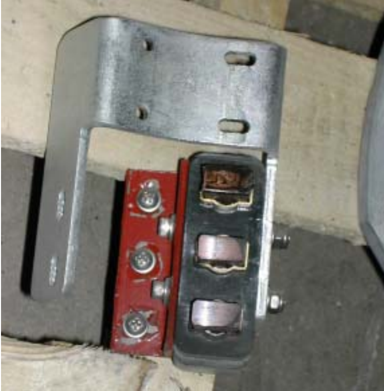
Figure D.12. The slip ring brushes. Note the grease on the top brush.
