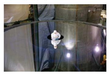
NSF provides the world's astronomers with two identical 8-meter telescopes in Hawaii and Chile, known as the Gemini Observatory. Shown here is the mirror of the telescope at Mauna Kea, Hawaii. The telescope is optimized for observations in infrared light. The thin mirror
