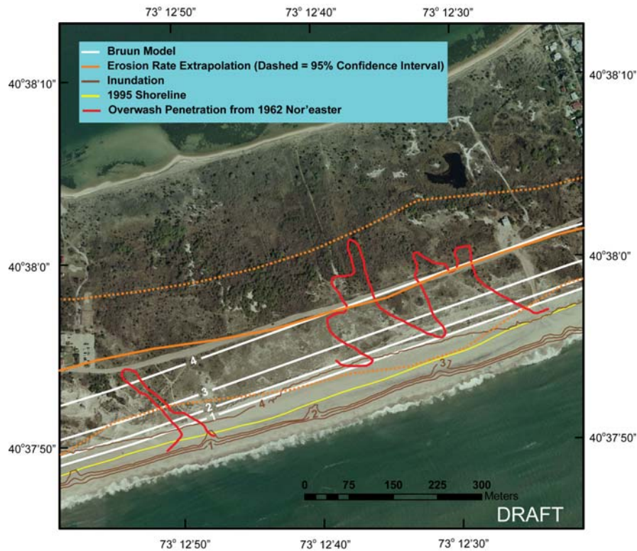
15106 15107 Figure H.5 Site 1 comparison of shoreline change projections for a portion of Fire Island, NY (See Figure 15108 H.1 for location). Aerial photograph obtained from the state of New York. 15109
