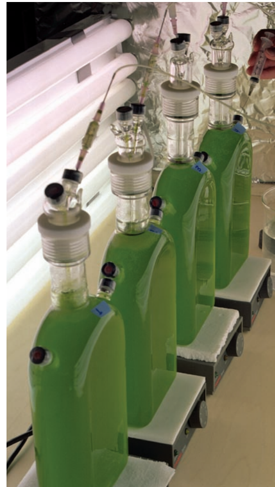
A set of bioreactors used for photobiological hydrogen production by green algae. PIX 08740
