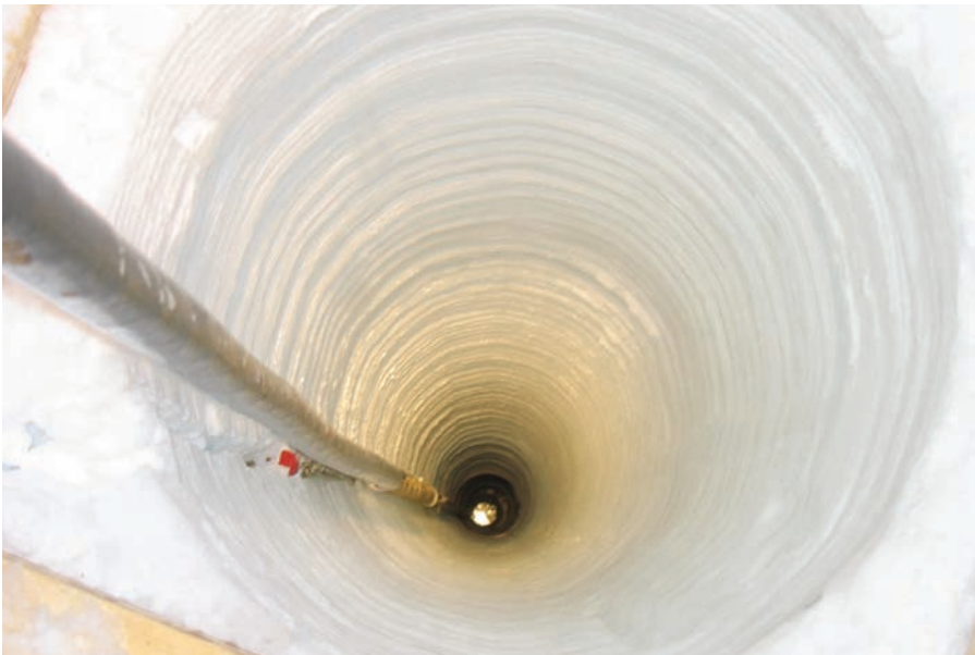
View of signal cables from strings of Digital Optical Modules extending down into the ice. Elusive particles, called neutrinos, will be detected arriving from distant astrophysical sources and carrying information about those sources, just as rays of light reveal objects to conventional telescopes.
