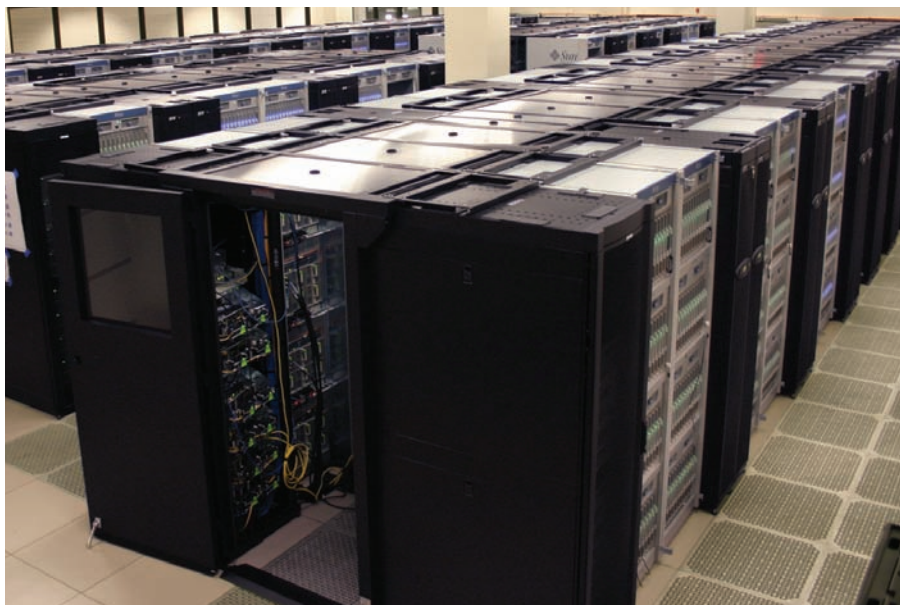
The "Ranger" supercomputer at the Texas Advanced Computer Center (TACC) will provide unprecedented computational capabilities—504 teraflops peak performance, 125 terabytes memory and 1.7 petabytes disk—to the national open science research community. This system represents a unique opportunity to explore the challenges of petascale science from science and technology perspectives.
