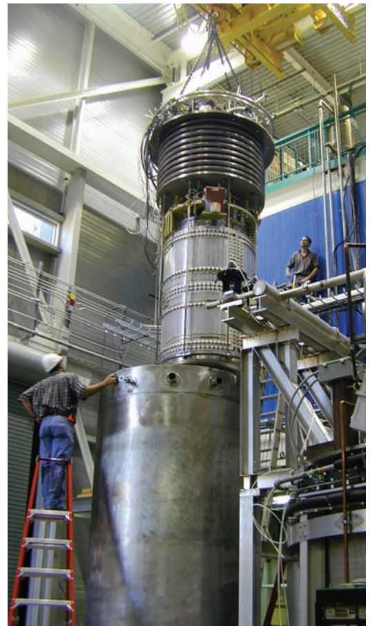
NHMFL technicians replace a coil for the Magnet Lab's world-record 35 Tesla all-resistive magnet.
