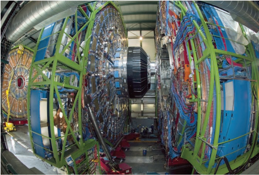
This image shows the CMS detector at the European Organization for Nuclear Research (CERN). The detector is 15 m diameter, 21.5 m long and weighs about 12,500 tons.
