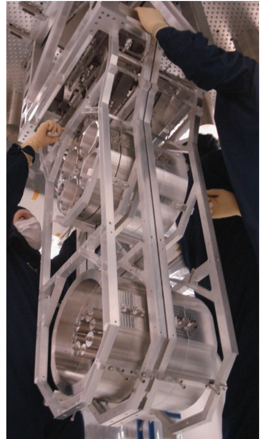
Engineer Stephany Foley of MIT LIGO is aligning the elements of a prototype test mass suspension for the planned Advanced LIGO Gravitational Wave detector. In this prototype, the cylindrical mirrors are replaced with metal pieces to allow testing on a less fragile system. It is suspended from an optics table on an Advanced LIGO seismic isolation system.
