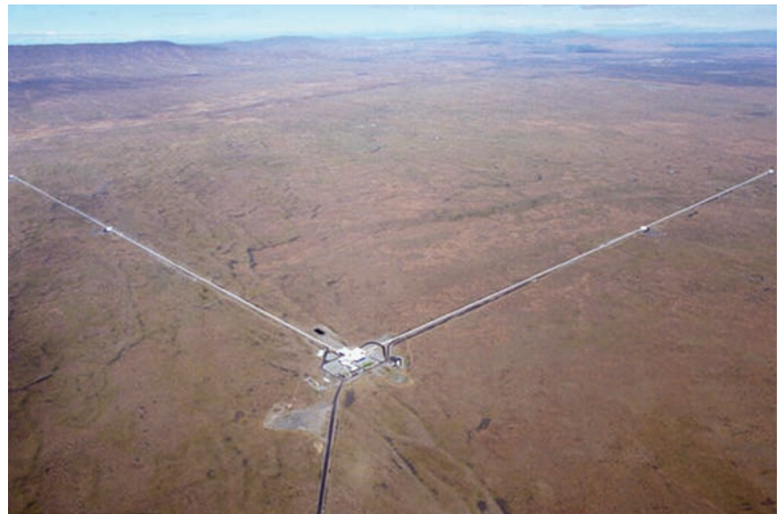
Aerial view showing the twin 4-km long arms of the interferometer at the Hanford, Washington, LIGO site.
