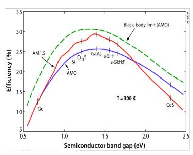
has been already been surpassed with innovative (not cheap) cells. Efficiencies > 40% have been attained, often with concentrators requiring two-axis suntracking and active cooling.
