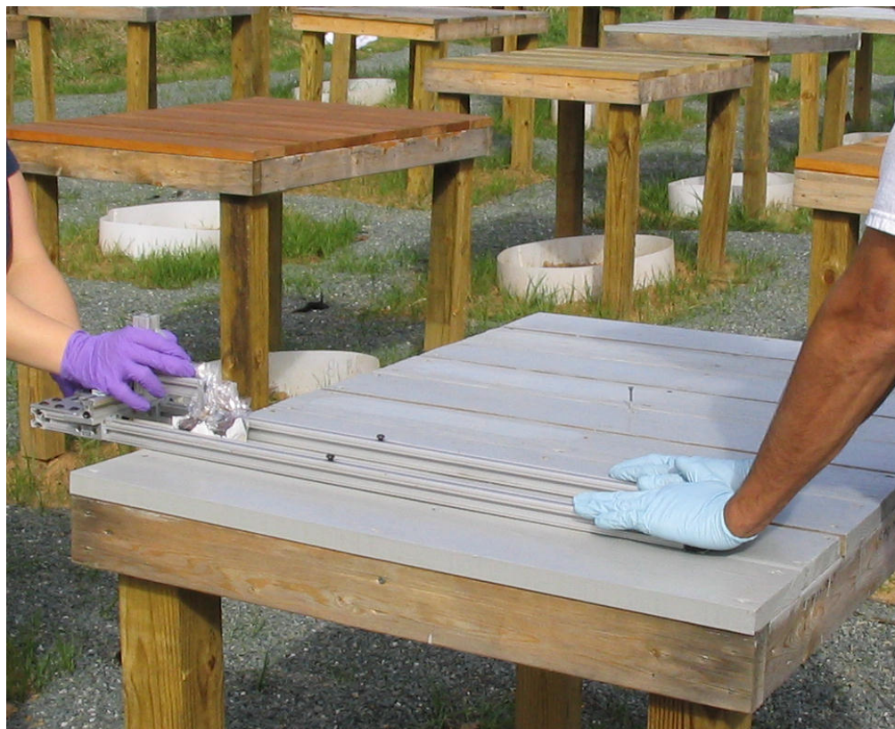
Figure 2-9. CPSC Wipe Sampling Apparatus
