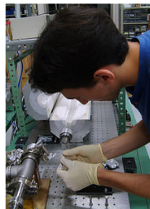
NanoJapan participant loads a sample into a CVD chamber at the University of Tokyo. Credit: Dvir Kafri.
