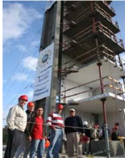
NEES investigators at UCSD's Seven Story Test Model. Credit: Prof. Jose Restrepo, Department of Structural Engineering, University of California at San Diego.
