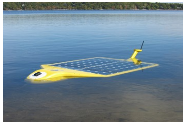
The new solar-powered autonomous underwater vehicle (SAUV-II) will be used for a variety of environmental monitoring tasks. Credit: Arthur C. Sanderson and D. Richard Blidberg.
