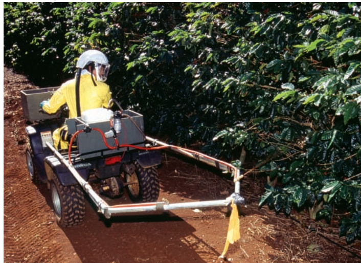
Technician Russell Ijima uses an all-terrain vehicle to apply a band of protein bait spray (containing spinosad) in a Hawaii coffee field.
