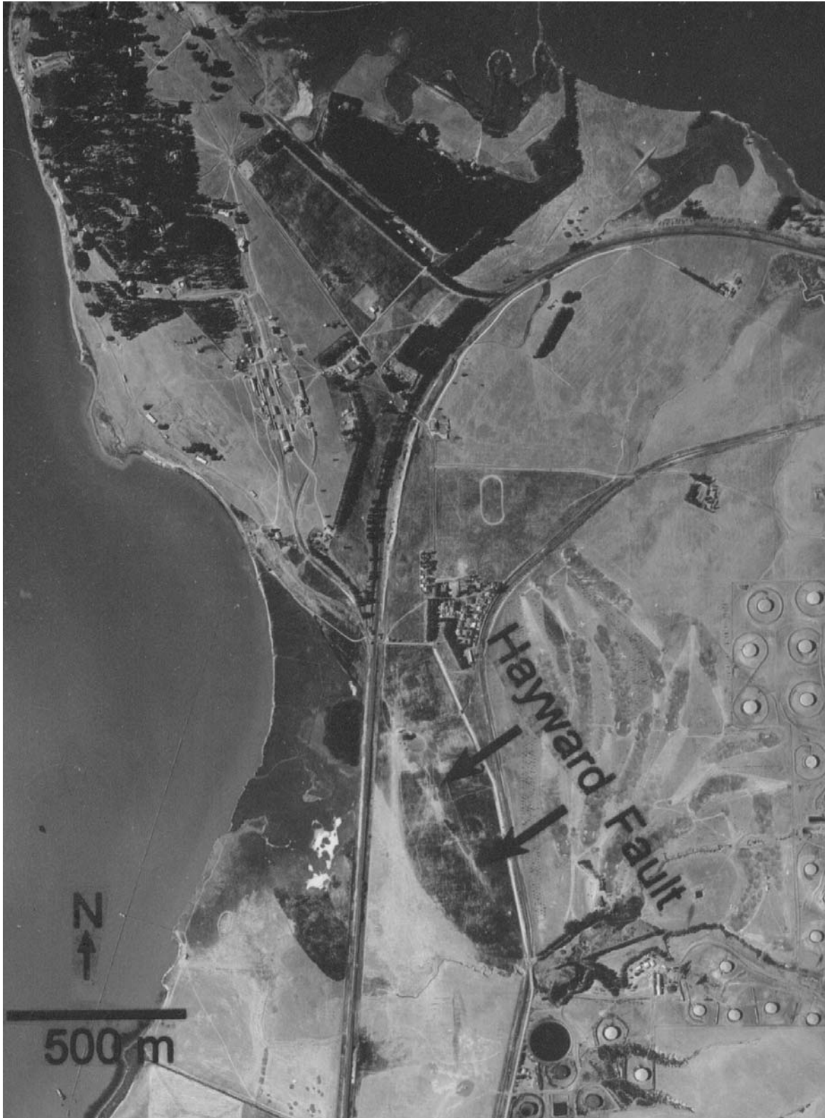
Figure 22. 1939 aerial photo showing the white linear feature that marks the location of the Hayward fault through what became Parchester Village in 1950. The white streak is the result of cultivation and erosion of an “E” soil horizon, which formed as a result of the water barrier produced by the fault. Most of the buildings seen here have been removed from the park.
