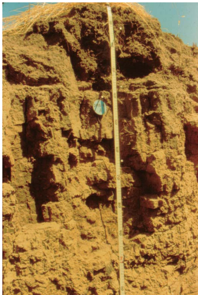
Figure 25. Moderately strong soil developed on the SW side of the Hayward fault in Trench DMG-E (Borchardt, 1988a).
