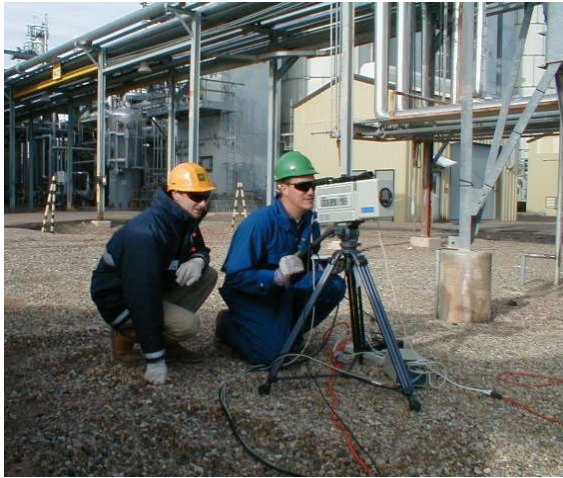
Handheld infrared remote imaging spectrometer for fugitive gas leak detection.
