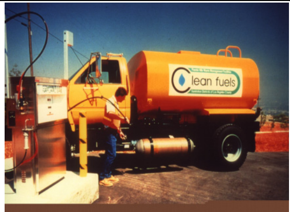
Landfill gas to compressed natural gas vehicle refueling station, Los Angeles, California
