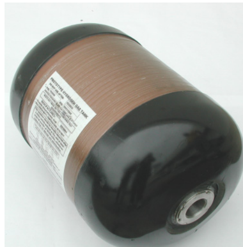
High-pressure, all-composite gaseous hydrogen storage cylinders encourage commercialization of hydrogen gas-powered vehicles.
