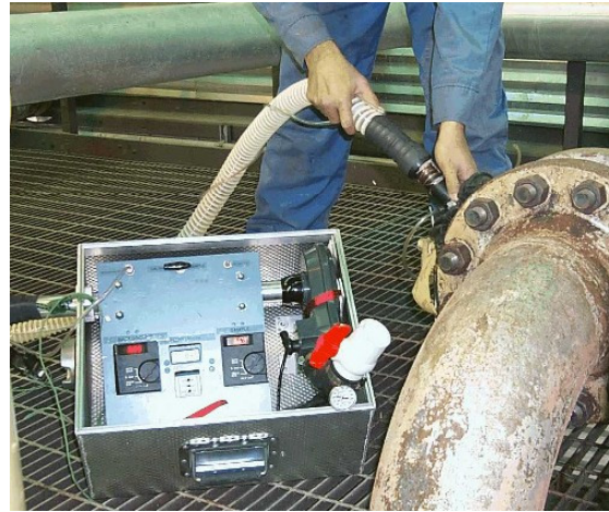
Hi-Flow™ Sampler to measure emission rates.
