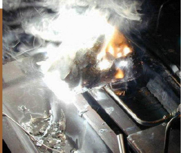
Figure 2. Molten Mg without protective cover gas.
