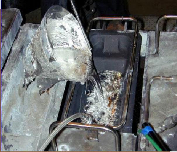
Figure 1. Molten Mg with SF 6 cover gas.
