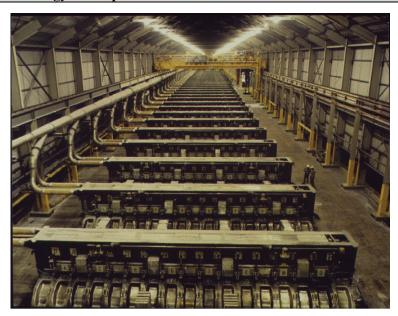
Primary aluminum production is the largest source of emissions of perfluorocarbons in the United States. Mitigation technologies and measures cannot only reduce emissions, but they also can improve process efficiency. (Reprinted with permission of Greenleaf Publishing.)
