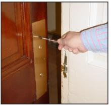
Figure 4: Testing restroom door weight
