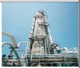
Nitric-acid plant controls for  $NO_x$  using both nonselective catalytic reduction and selective catalytic reduction technologies. Nonselective catalytic reduction is very effective at controlling  $N_2O$ .
