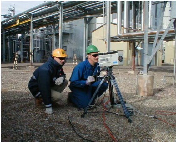
Handheld infrared remote imaging spectrometer for fugitive gas leak detection.
