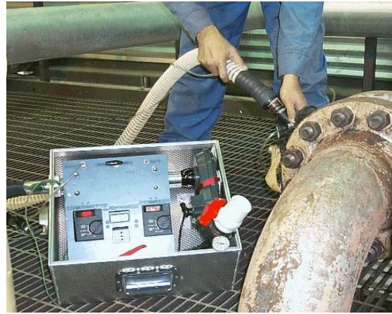
Hi-Flow™ Sampler to measure emission rates.
