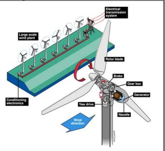
wind plants range in size up to several megawatts, and smaller turbines (under 100 kilowatts) serve a range of distributed, remote, and stand-alone power applications.
