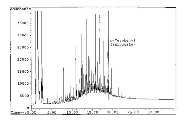
FIGURE 3  ${\rm EXAMPLE~CHROMATOGRAM~OF~A~30~PPM~DIESEL~STANDARD~WITH~THE~} \\ {\rm BASELINE~PROJECTED~BETWEEN~C_{10}~AND~C_{28} }$
