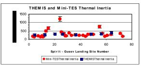
**Figure 2.** Plot comparing the thermal inertia trends between THEMIS-derived thermal inertia from orbit and Mini-TES-derived thermal inertia of the surface at the MER-Spirit landing site.
