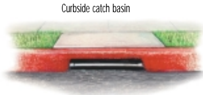
Curbside catch basin
