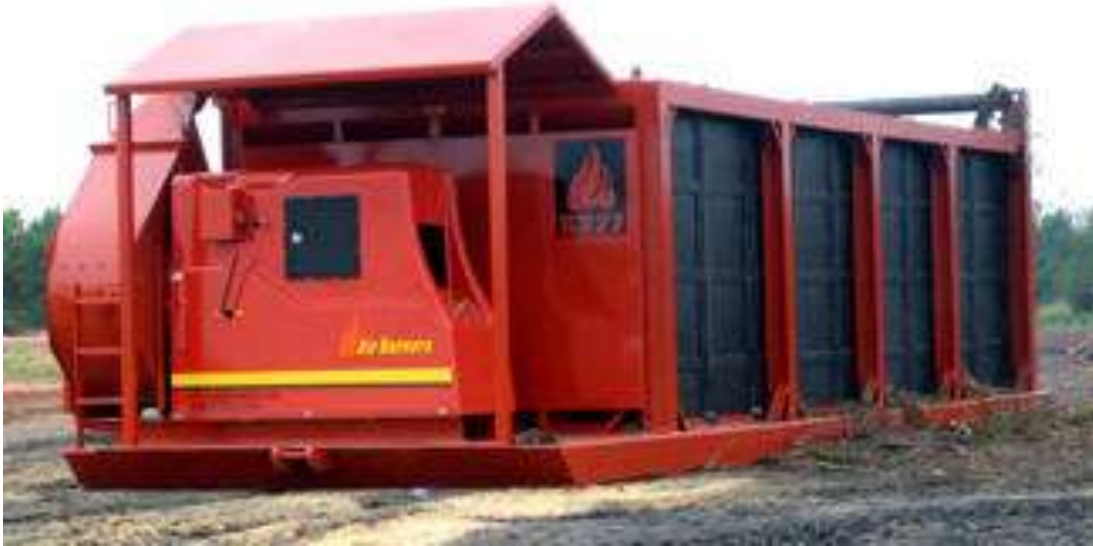
Figure B-1. Configuration of a Typical Air Burner (ABT) Unit
