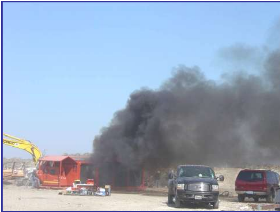
Figure A-6. Smoke plume generated during initial stage of startup due to premature combustion prior to start of air curtain. Amid Landfill (October, 25, 2005).
