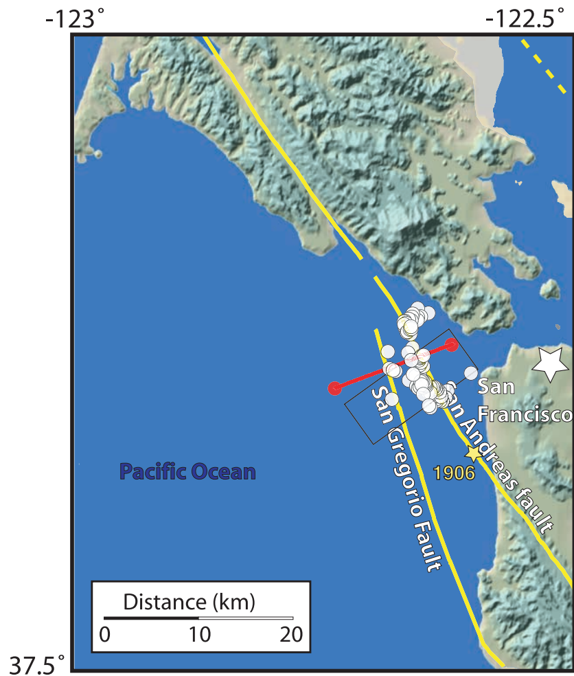
Figure 1. The San Gregorio fault approaches the more northwest trending San Andreas fault in the offshore Golden Gate region. The red line shows the location of a seismic refraction and reflection cross-section model. The white dots are a subset of relocated earthquake epicenters [Waldhauser and Ellsworth, 2000] that occurred near the seismic cross section. The black box around the epicenters shows the area of hypocenters collapsed onto the 2-D cross section in Figure 2. The yellow star shows the approximate epicenter of the 1906 earthquake [Geist and Zoback, 1999].
