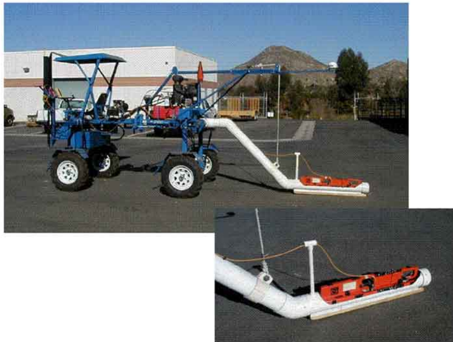
Figure 3. Mobile GPS-based electromagnetic induction (EMI) equipment showing (a) a side view of the entire rig and (b) a close-up of the sled holding the EMI unit.
