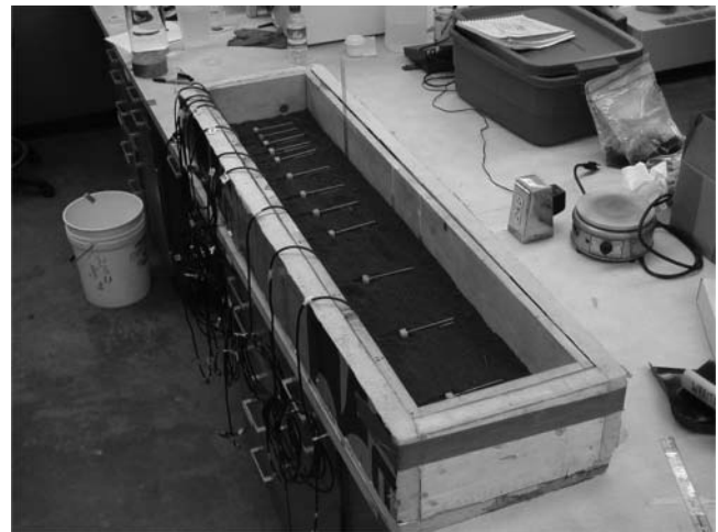
Fig. 4. Insulated soil container with 12 probes for evaluation of multiplexer-induced signal interference under variable probe spacings and soil water contents.
