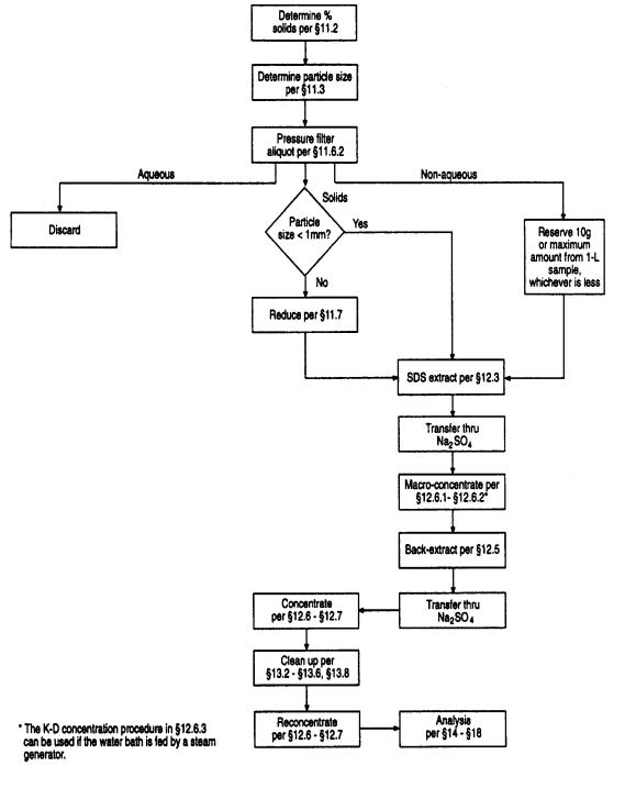
Figure 2. Flow Chart for Analysis of Multi-Phase Samples
