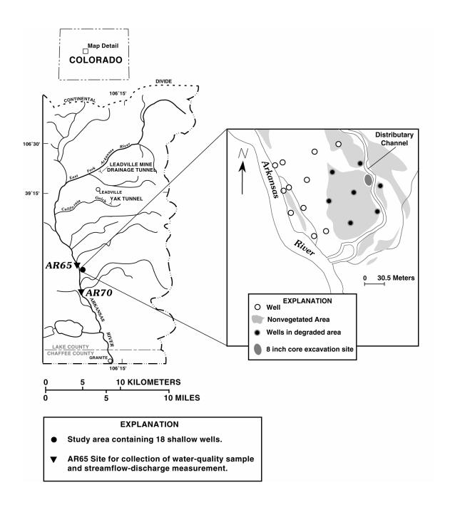
**Figure 1.** Schematic of the study site showing the main study area where shallow ground water wells were installed and surficial materials collected. Also shown are the excavation site of the 8-inch-diameter core, and the upstream and downstream sampling sites along the Arkansas River.
