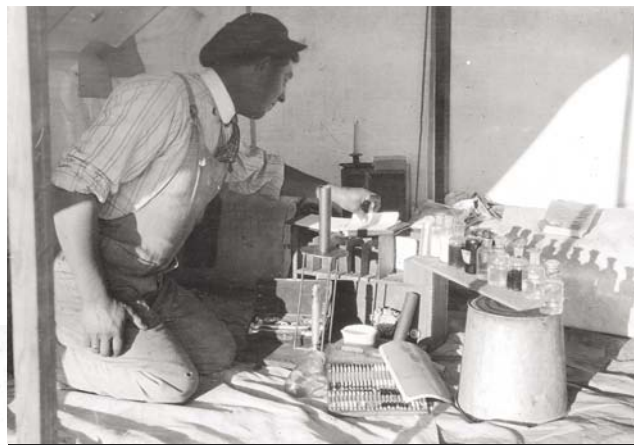
Portable analytical equipment was transported by wagon in 1907 to help determine the distribution of elements while conducting field work in Montana. The analyst could perform wet chemical analyses in a tent when camp was established. (From Taggart, 1995; R.W. Stone, photographer.)
