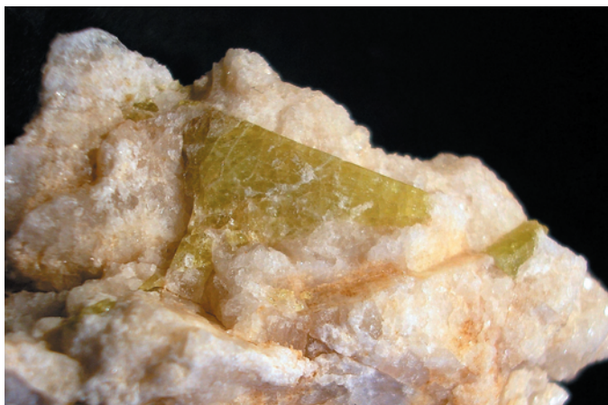
Figure 19. Platy crystals of yellow-green chrysoberyl in feldspar-rich pegmatite from the Taglo Mine at sample site AP-058. The largest crystal in this image is about 1.4 cm across.
