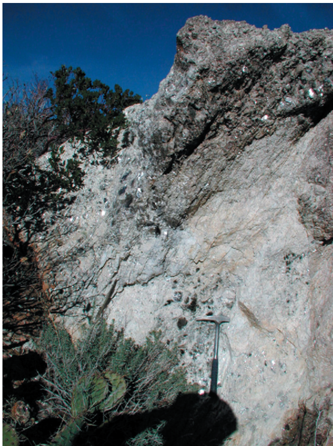
Figure 18. Detail of 1.5-m-wide pegmatite at sample site AP-058, Taglo Mine, showing coarse muscovite books in the border zone of the dike (bright areas at top of view).
