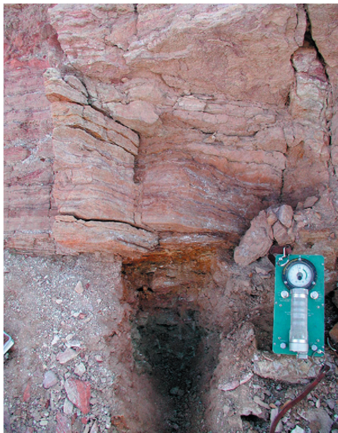
Figure 24. Radioactive clay-altered tuff (in dug-out area) beneath limestone, Long Shot Mine. Scintillometer, about 25 cm long, for scale.
