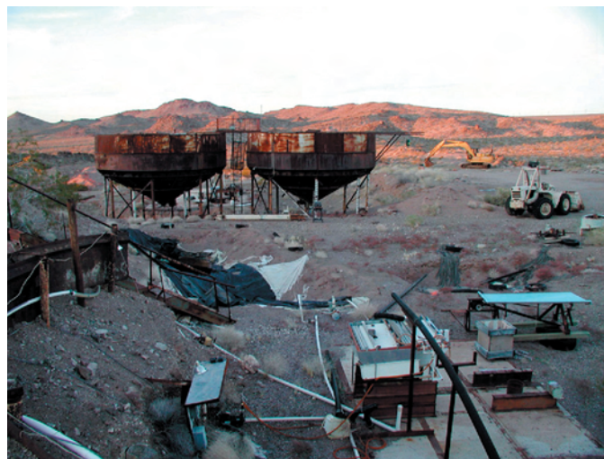
Figure 37. Remains of a mill near the site of sample AP-051. The small blue shaking table at right suggests that gravity recovery of gold was planned. The mill appears abandoned, but the presence of modern excavation equipment indicates recent activity.
