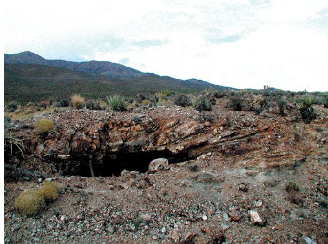
Figure 40. Shallowly-dipping sheared, altered, and mineralized zone southwest of the Silver Bell Mine. AP-024C is a chip sample taken from the hammer (right of opening) downward 1.2 m across the sheared and limonitic rock to the top of unoxidized greenish gneiss below.
