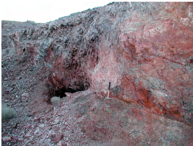
Figure 36. Small open-pit mine with old underground working along north-dipping fault. Sample AP-051 was collected from the shattered zone below the hammer.
