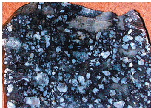
Figure 14. Fine-grained porphyritic phase of upper unit of the Searchlight pluton. Sample 4-033102 contains about 58 percent \text{SiO}_2 (Ludington and others, 2005). Image is approximately actual size.
