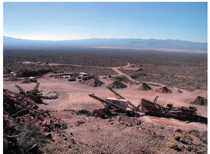
Figure 52. Crushing and screening equipment with light pink to purplish-gray decorative stone stockpiled at the Lucky Dutchman Mine, Crescent district.
