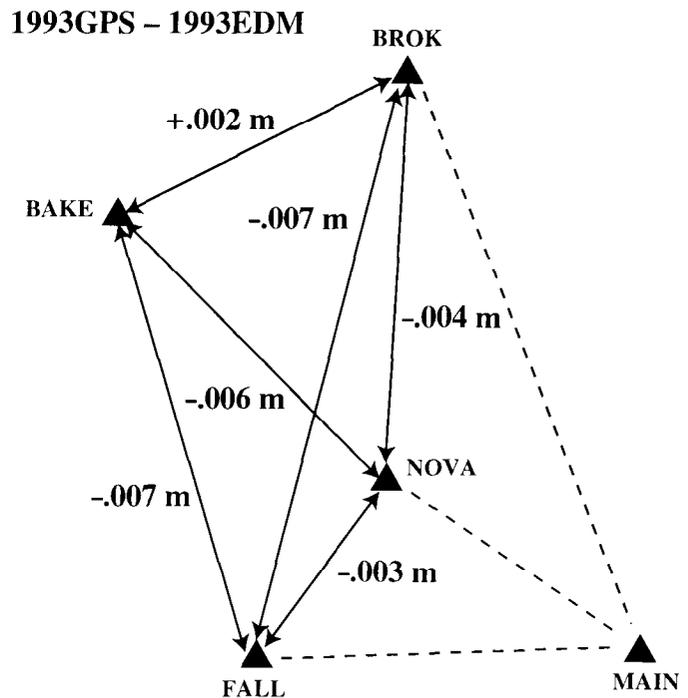
**Figure 4.** Novarupta line-length differences for 1993 GPS and 1993 EDM surveys.
