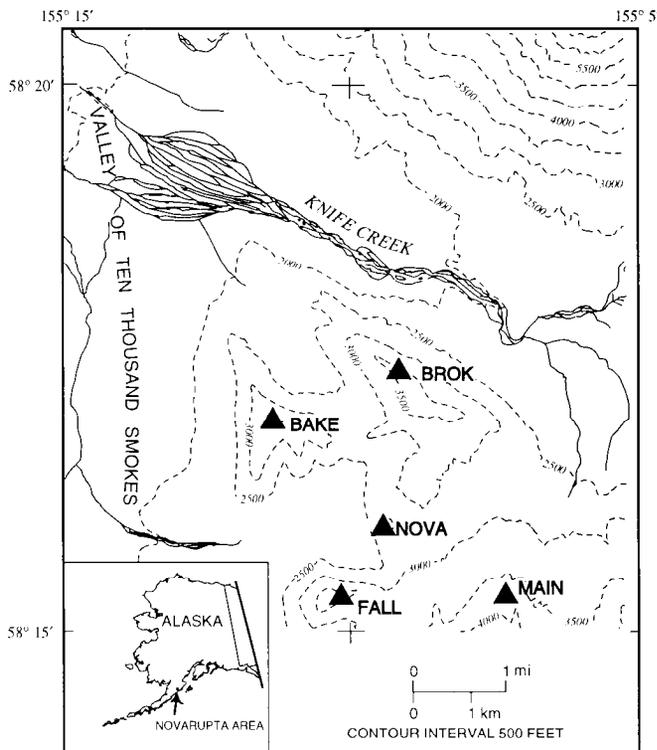
**Figure 1.** The braced quadrilateral geodetic network in the Novarupta area of the Valley of Ten Thousand Smokes. Benchmark locations are indicated by triangles and abbreviated names used in the text.
