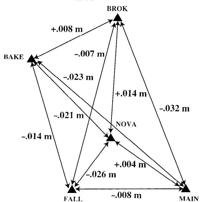
**Figure 6.** Novarupta line-length differences for 1995 GPS and 1993 EDM surveys.
